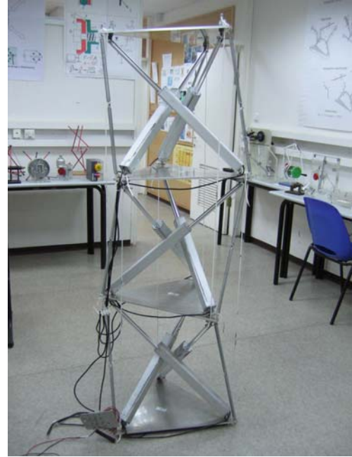
Figure 6. Deployable tensegrity structure. This structure was developed at the adjustable deployable tensegrity structure lab at Tel Aviv University.
